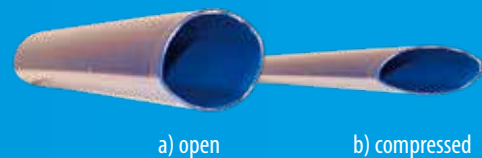
The two extreme deformation conditions of the hose.
