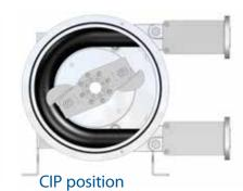
PT pumps are available in "CIP wheel" (Clean In Place) option. It allows users, by simply reversing the direction of rotation of the pump ( $\frac{1}{2}$  turn), to be able to retract the shoes automatically, in order to make the cleaning and sterilization operations, without any action on the pump. The client saves time and will keep the highest level of functionality in the process.
