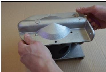
Fig. 3.7.2 Lay down the pump on one side and lift one of the housings [11].
