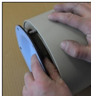
Fig. 3.7.5 Unscrew the diaphragm [15] from one side of the pump.
