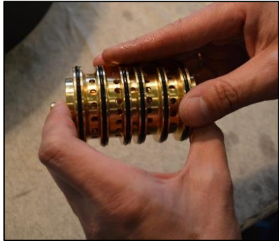
Fig. 3.6.2 When putting the air valve [61] into the centre block [12], apply some water or alcohol on the O-rings to provide smooth insertion of the air valve. It is recommended to use a pressing device for this operation. ATTENTION! When inserting the TX25 size air valve, replace the shaft with a screw and a nut to make sure the air valve assembly remains properly fastened.
