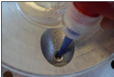
Fig. 3.6.4 Apply some Loctite 243 on the thread before screwing in of the valve ball stops [22]. ATTENTION! Make sure the glue is inserted on the thread and not only on the bottom surface of the orifice.
