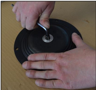
Fig. 3.6.5 When assembling the diaphragms [15], the first step is to screw the grub screw into one of the diaphragms as much as possible.
