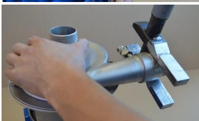
Fig. 3.5.8 Unscrew the connection adaptor [1364].
