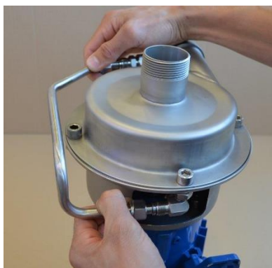
Fig. 3.5.6 Remove the metal pipe [1363].
