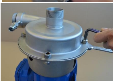
Fig. 3.5.11 Unscrew the casing mounting screws [141] and remove them with the nuts [143] and washers [142].
