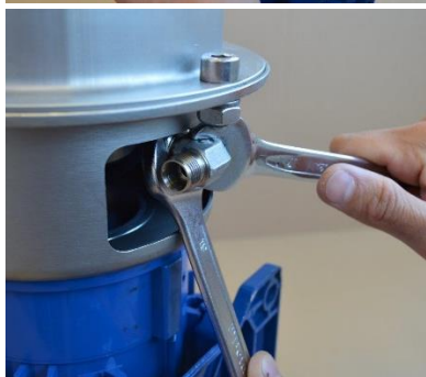
Fig. 3.5.7 Unscrew and remove the elbow union [1367].
