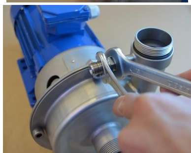
Fig. 3.5.10 Unscrew the straight union [1366].
