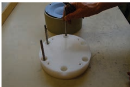
Fig. 2.4.5. Take the pin screws [14] out of the dampener housing [11].
