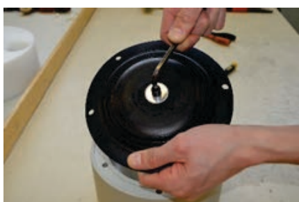
Fig. 2.4.7. Using an allen key, unscrew the shaft ending [1652] from the diaphragm.
