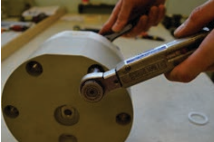
Fig. 2.5.11. Tighten the nuts [37] cross-side by means of a torque wrench with the appropriate torque (see chapter 4.2.).
