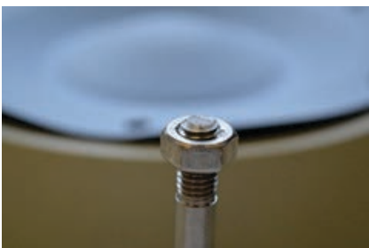
Fig. 2.5.8. Screw the nuts [37] onto the pin screws [14] so that ca. two threads are visible over the nut.
