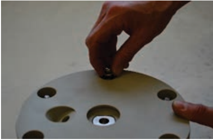
Fig. 2.5.10. Insert the washers [38] and nuts [37] on the pin screws [14] from the side of the block and pre-tighten the nuts cross side.
