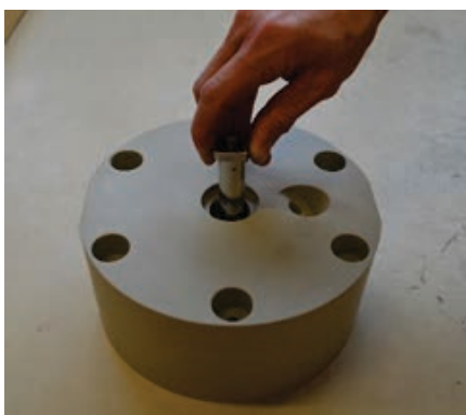
Fig. 2.4.8. Push out the shaft [1651] from the dampener housing.
