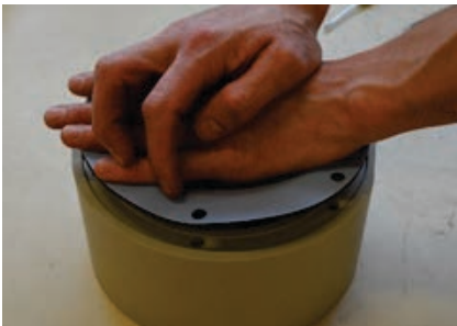
Fig. 2.5.6. Push the diaphragm [15] in, so that it is touching the dampener block [12].
