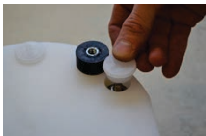
Fig. 2.4.2. Remove the nut covers [579] from the dampener housing and block.
