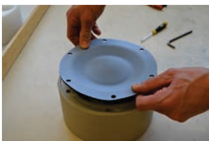
Fig. 2.4.6. Unscrew the diaphragm [15] by hand (clockwise).
