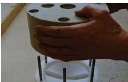
Fig. 2.5.9. Turn over the dampener housing [11] and insert the dampener block [12] onto the pin screws [14].
