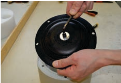
Fig. 2.5.4. Screw the shaft ending [1652] into the diaphragm [15].
