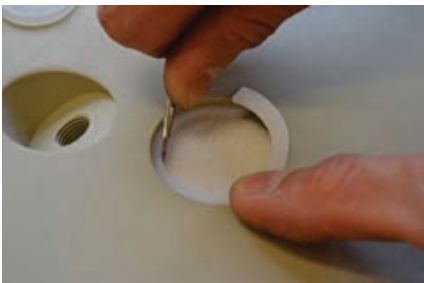
Fig. 2.5.13. Insert the muffer [25] and the circlip [27] in a circular manner.
